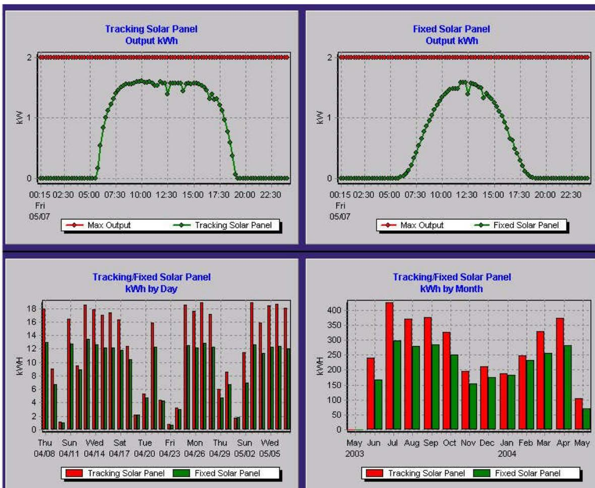
So if you were to take identically sized modules and test one on a fixed mount and one on a dual axis tracker you would see 30 to 45% more electricity over the course of a year.
